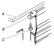
A. Countertop B. Retaining bracket C. Mounting screw (provided)
